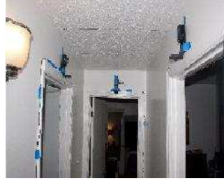
Fig. 4. Height sensors deployed above doorways in a home.
