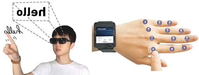
Figure 1: Harness vibrations for finger tapping and writing systems with commodity smartwatches.
