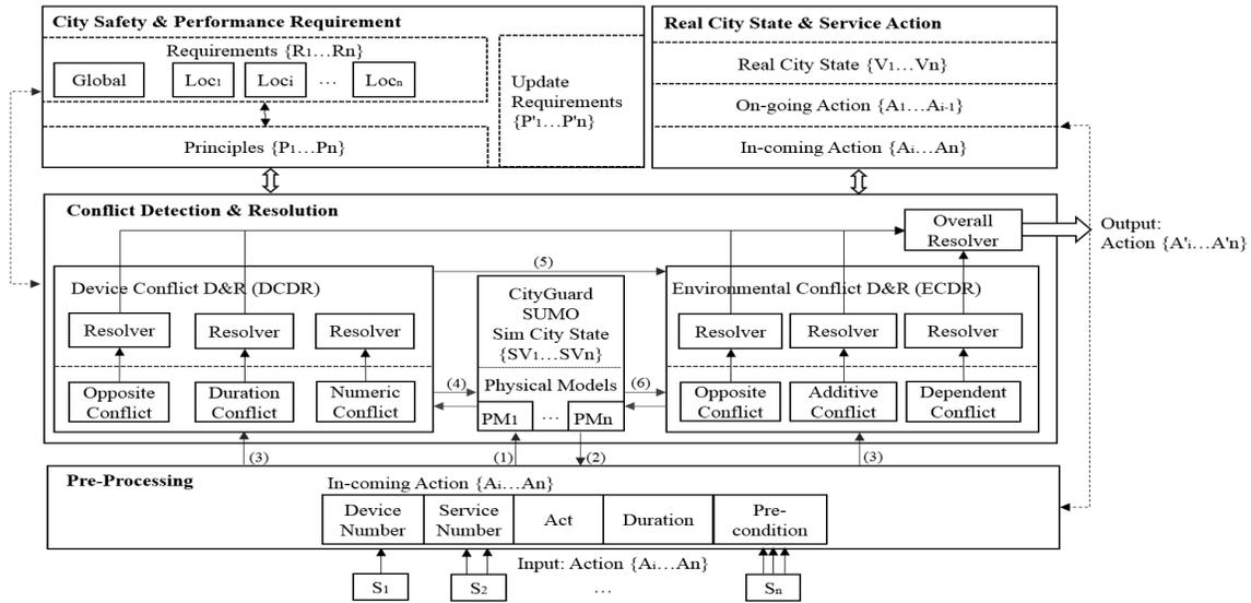
**Figure 3: CityGuard Structure** (*Pre-Processing* intercepts and checks the safety of the single action, *Conflict Detection & Resolution* detects conflicts among actions after Pre-processing, and *City Safety & Performance* and *Real City & Service Action* store the safety requirements and city states, respectively. Section III describes each component in detail.)
