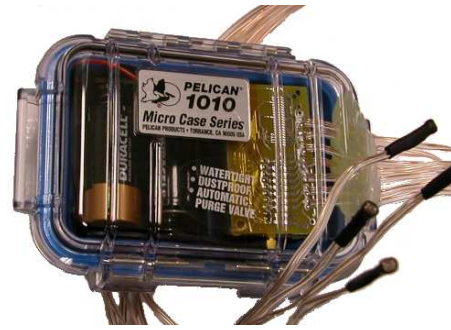
Figure 9. Packaged “Medusa” sensor module.
