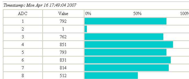
Figure 2. LUSTER web server generated page reporting ADC levels for a pre-selected remote sensor node.
