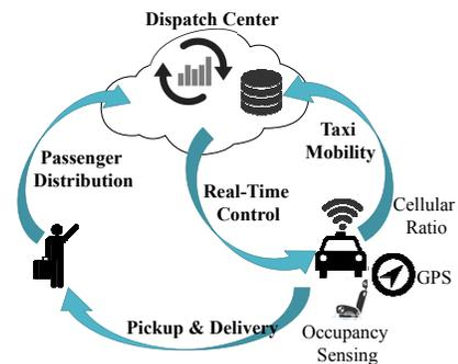
Figure 1: A prototype of the taxi dispatch system
