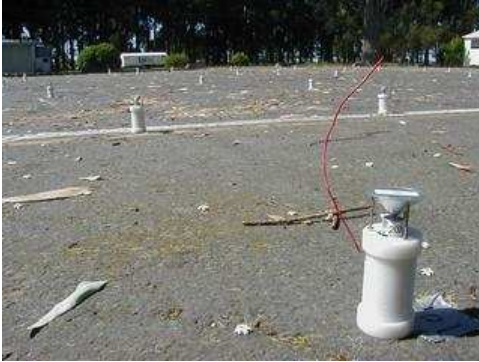
Figure 11: Final Deployment The final deployment involved 49 nodes over a 13x13m area on a paved surface.
