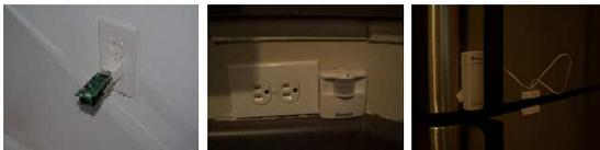
**Fig. 5.** Motetrack tags and beacons (left) were used to collect ground truth locations. Motion and magnetic reed switch sensors (middle/right) were used to evaluate STAR.
